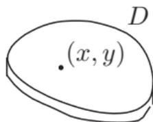
$$u_t(x, y, t) = c(u_{xx}(x, y, t) + u_{yy}(x, y, t)), \\ (x, y) \in D, \quad t > 0$$
