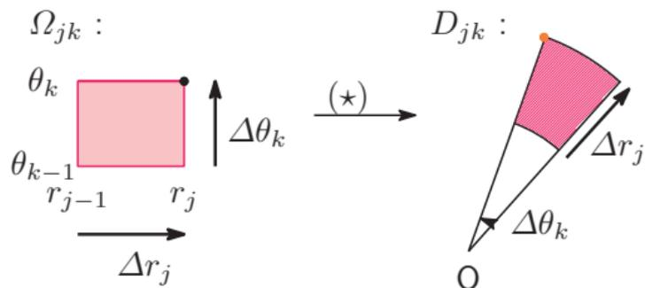
$$m(D_{jk}) = r_j \Delta r_j \Delta \theta_k - \frac{1}{2} (\Delta r_j)^2 \Delta \theta_k \doteq r_j \Delta r_j \Delta \theta_k$$
