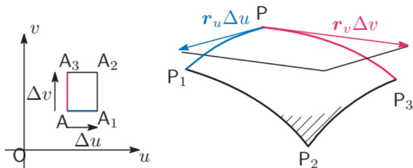
$$\begin{aligned}\overrightarrow{PP_1} &= \vec{r}(u + \Delta u, v) - \vec{r}(u, v) \doteq \vec{r}_u(u, v)\Delta u, \\ \overrightarrow{PP_3} &= \vec{r}(u, v + \Delta v) - \vec{r}(u, v) \doteq \vec{r}_v(u, v)\Delta v\end{aligned}$$
