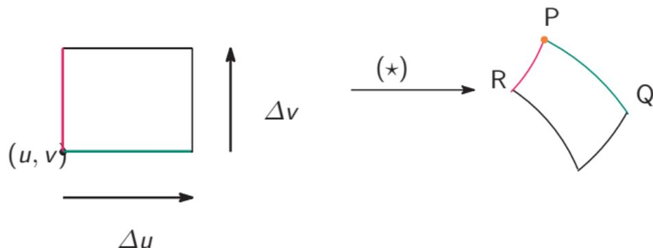
$$\begin{aligned} \overrightarrow{PQ} &= (\varphi(u + \Delta u_j, v) - \varphi(u, v), \psi(u + \Delta u_j, v) - \psi(u, v)) \\ &\doteq (\varphi_u(u, v)\Delta u_j, \psi_u(u, v)\Delta u_j) = (\varphi_u(u, v), \psi_u(u, v))\Delta u_j \end{aligned}$$
